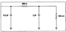
HP 16517/18A Probe load equivalent circuit.
